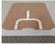
Step 3: Insert Support Handle (B) into the pre-assembled base plate (A), pressing in snap button and snap bolt. Ensure that both snaps are fully extended through holes. Secure safety nut to fully extended snap bolt with wrench (C.)
