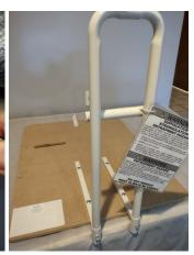
Step 3: Insert Transfer Handle into the base plate (A), pressing in snaps. Ensure that both snaps are fully extended through holes. Secure 7/16" safety nut to fully extended snap bolt with wrench (C.)
